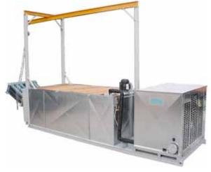
These plants are assembled on a skid ready to operate, except for the overhead crane and can filler.
